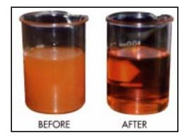
can break up the body of water into small droplets, which become dispersed in the oil. Water finely dispersed or emulsified in the oil becomes practically impossible to separate by gravitational means.
