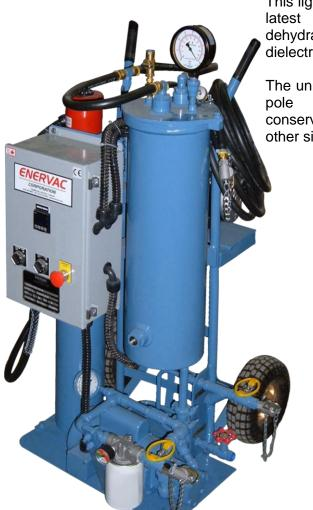
This lightweight Mini Degasifier cart uses the latest high vacuum technology to filter, dehydrate and degasify insulating and dielectric fluids.
